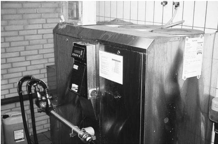
Fig. 1: Small 125 l. CIP-cleaning system for milking parlour and milk storage
