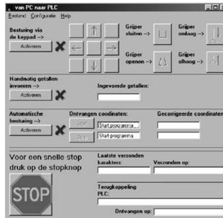
Fig. 4: Main screen of user interface PCPLC program for communication between PC and PLC
