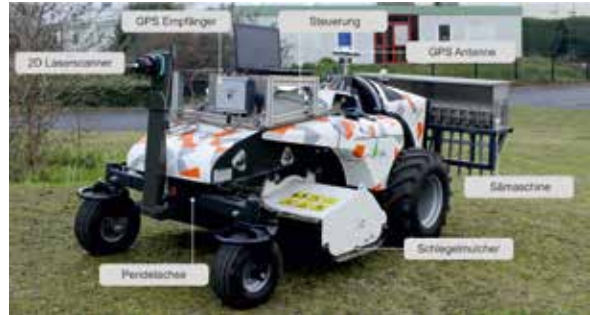
Abb. 2: Prototyp des Weideroboters Fig. 2: Prototype of the pasture robot
