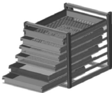
Fig. 4: Screen separator for forage (5 square type pan)
